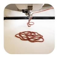
Tip: Unwind the ball of yarn/wool and splay out next to the machine, to ensure smooth feeding without tangling. Continually monitor the yarn/wool as it feeds.
